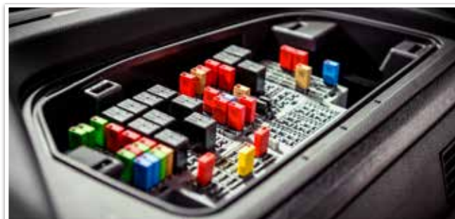
In-cab electrical panel
